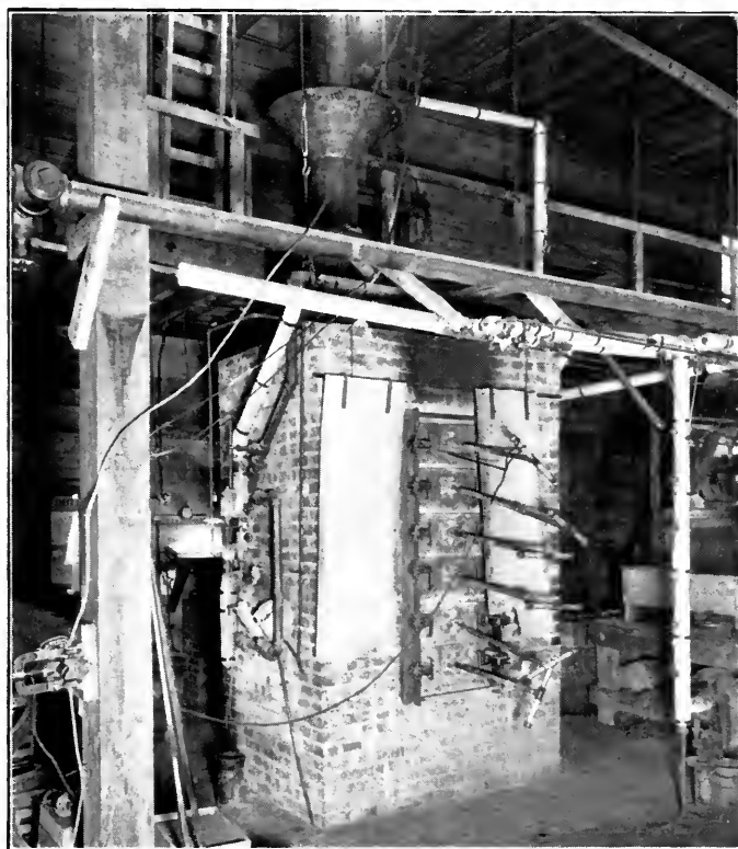
Upper Photo—The small Experimental Electric Furnace Developed for the Steam Activation of Charcoal. Lower Photo—Wedge Furnace No. 1, which was the first Horizontal Activator Developed.
